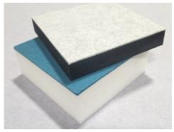
J2 Acoustic Polyboard Composite Panel is a sound absorbing polyester felt panel that consists of a 1 in 6.0 pcf density backer panel and a 3mm PET Felt Fabric Facing.
